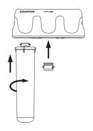
**NOTE.** There is no need to install a membrane cartridge at this point. To flush the RO-312S Pro, screw the flushing plug into the middle slot of the manifold block.
